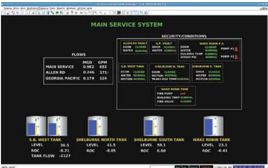
Main Service System SCADA Overview
